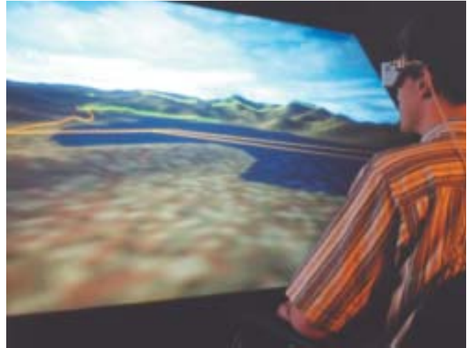
The Immersedesk, used for advance imaging and interactive applications, offers a three-dimensional view that changes when the user’s head moves.
