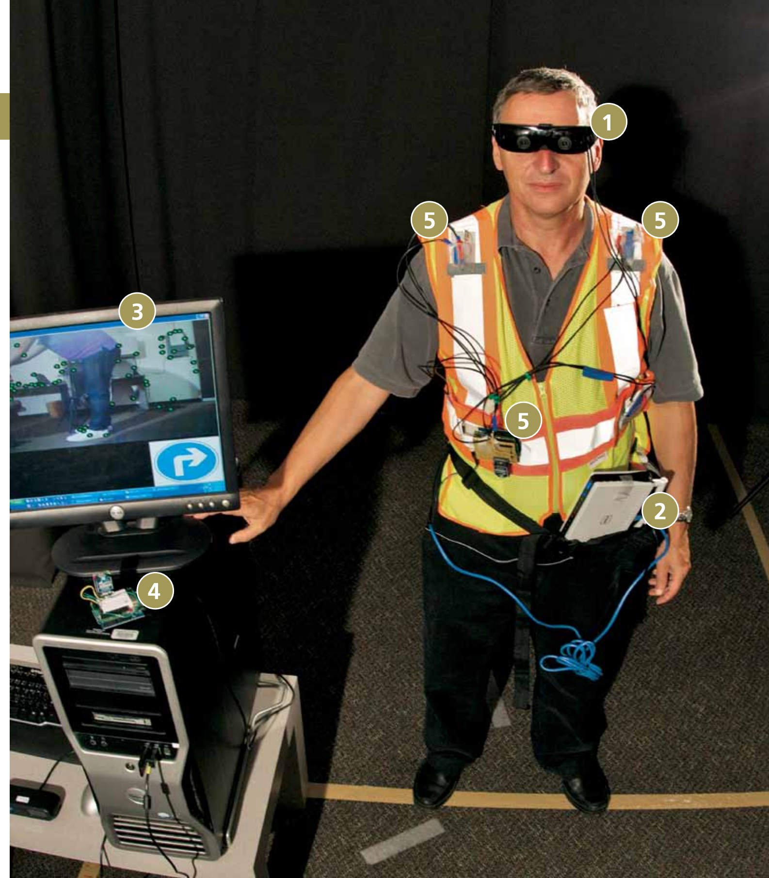
HOW IT WORKS—GUIDE VESTS FOR THE BLIND. 1 Some fancy glasses—the Vuzix WRAP 920 AR—see the world. Eye mounted cameras capture two separate images. 2 The images from the glasses are transmitted to the computer via wireless hub. 3 A computer fuses the two separate images together to create 3D information. A special algorithm—Simultaneous Localization and Mapping (SLAM)—is used to interpret the image, identifying a safe path through potential obstacles. 4 Based on this, the controller (atop the computer) sends a signal to the vest’s wireless receiver. 5 The wireless receiver talks to one of the vest’s four micro-motors (similar to cell phone buzzers), mounted on the shoulders and hips. If a shoulder-mounted motor vibrates—user should sidestep in that direction. If a hip mounted motor vibrates—user should change angle of their direction. If all four motors vibrate, that signals the user to turn around and go somewhere else.
