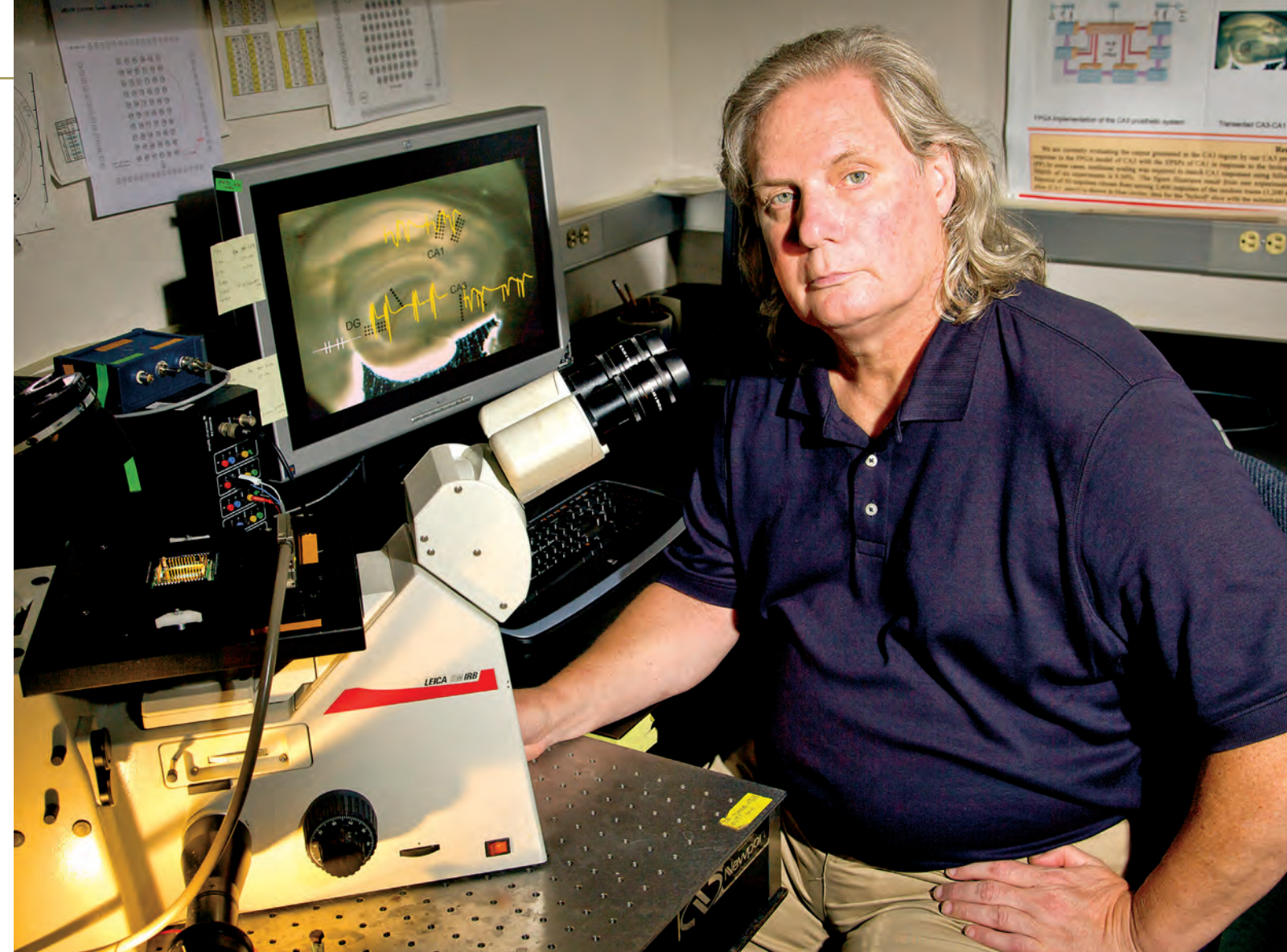
Ted Berger in his laboratory with a "conformal multi-electrode array system" designed to function as an interface between a living slice of rat brain tissue (shown on the video monitor) and microchip electronics (not shown). Such "neuron-silicon interfaces" are allowing biomimetic microelectronics to connect directly with the brain, and enabling them to serve as neural prostheses for the damaged brain.
