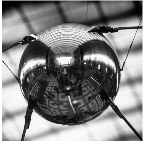
MAN'S STEP ON THE FIRST RUNG OF SPACE TRAVEL, THE SOVIET UNION LAUNCHED AN 184-POUND SPUTNIK VEHICLE LIKE THIS MODEL INTO EARTH'S ORBIT, OCTOBER 4, 1957. LEFT, PERIOD POSTER FROM JPL CELEBRATING EXPLORER I.
