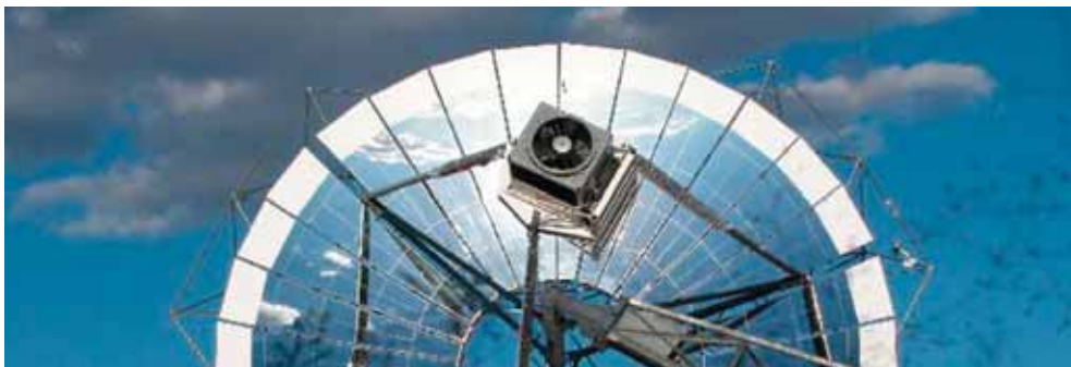
A dish system collects energy from the sun and concentrates it, producing heat that is transferred to a generator.
